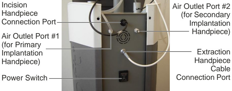
Figure 4-3. System Components (Upper Rear)
