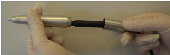
Figure 3-72. Inserting the Handpiece Body onto the Blade Holder
