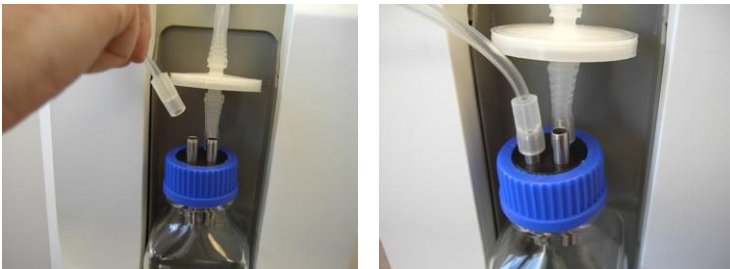
Figure 3-61. Connecting the Extraction Tube to the Jar
