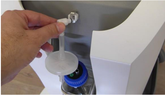
Figure 3-41. Connecting the Filter Assembly to the System's Vacuum Connector
