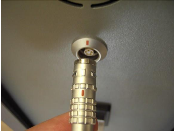
Figure 3-45. Aligning the Red mark of the Handpiece Cable Connector with the Red Mark on the Receptacle
